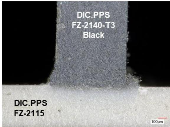
Pic. 2: Micrograph: The joining zone shows a good material mixing of the joining partners in the welding area.
