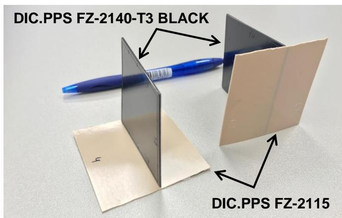
Pic. 1: Material samples are welded together in a so-called T-joint; in a test procedure created at DIC, the pull-off forces are determined and compared with other material variants.
